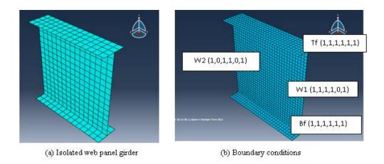
Fig. 2. Web panel girder used in analysis
