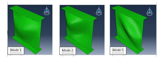
Fig. 5. Buckling modes of the web panel girder under shear force
