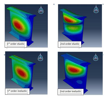
Fig. 7. Out of plane displacement contours for different analysis cases
