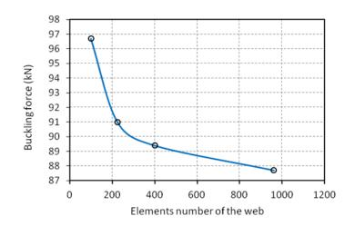
Fig. 4. Mesh size effect on buckling result for Mode 5
